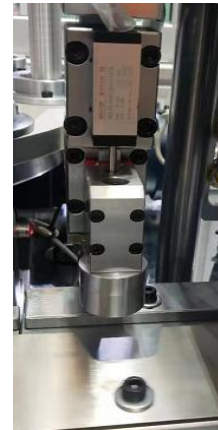
B shield pressing and checking
