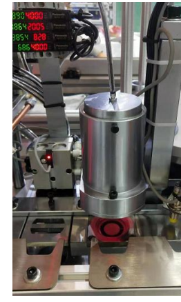
Fibre optical check on grease
