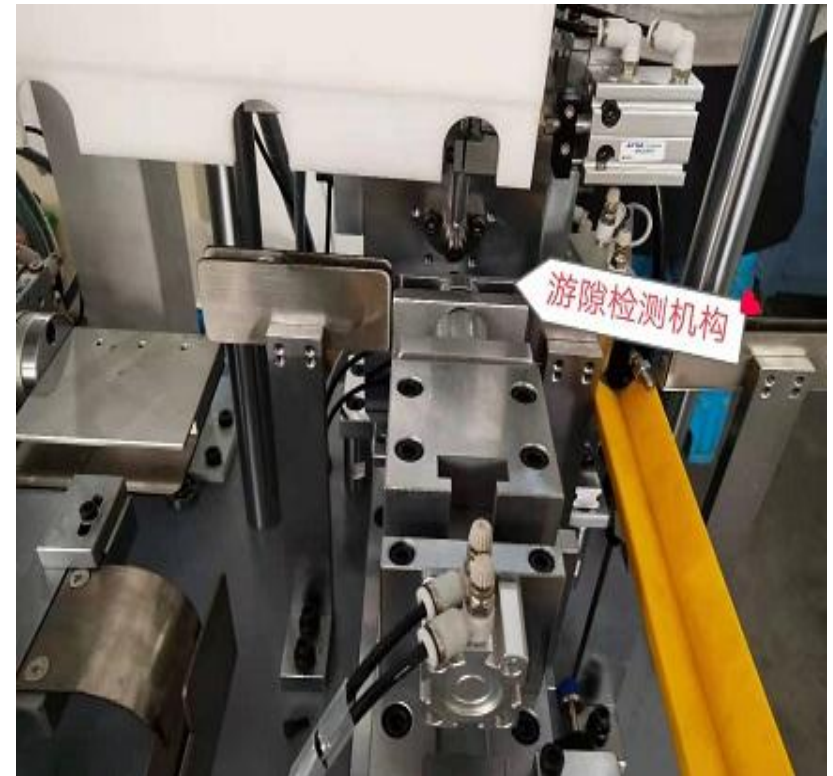
Radial clearance checking
